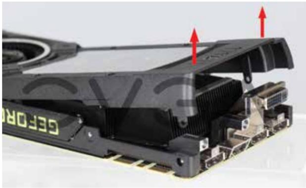
5) Now remove the heatsink and set it aside. We suggest cleaning the bottom of the heatsink, as the thermal compound left there can smear and spread.
