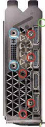
1) First remove the bracket by removing the 5 screws on the bracket, the perpendicular screw holding the bracket to the PCB, and the 2 standoffs on the DVI port. (#1 Phillips bit)
