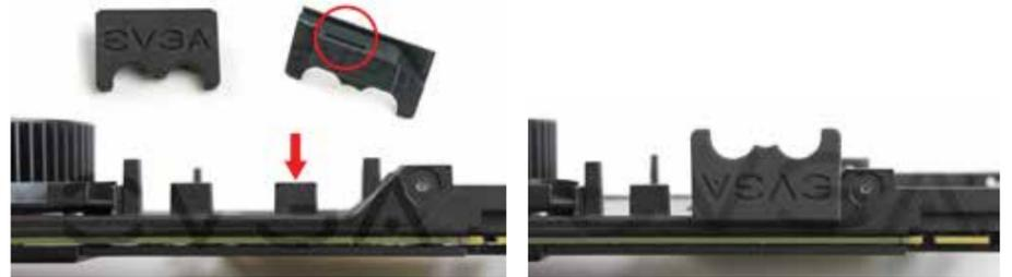
11) Remove the plastic cap on water block, use the 4 Spring Screws previously removed to mount the block on the GPU (Thermal compound is pre-applied to the block).
