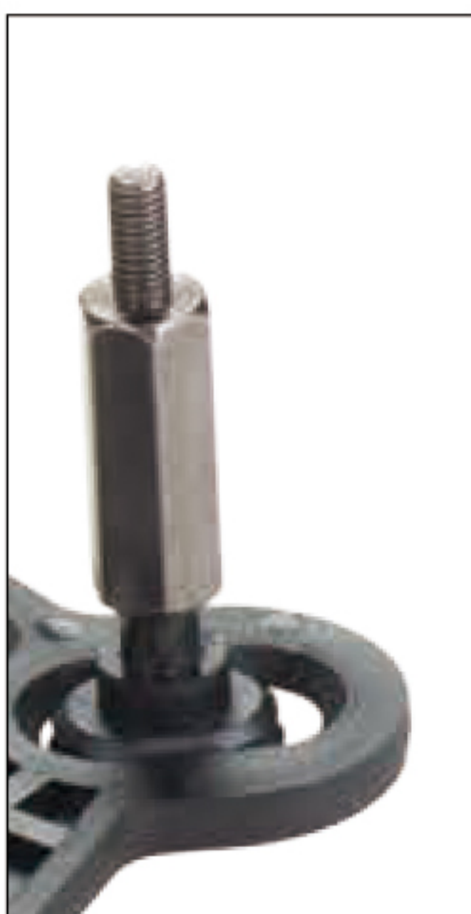
a. Screw standoff base into backplate. A B or C
