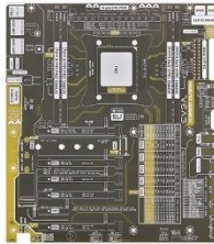
Baseplate with Visual Aids Study platform for pre-testing and platform troubleshooting. Has handy printout of the X299 DARK components, PCIe mapping and other helpful information.
