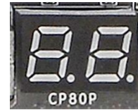
Debug LED with CPU Temperature Monitor
