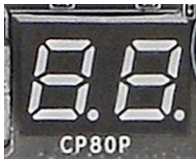
Debug LED with CPU Temperature Monitor
