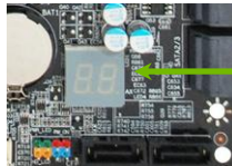
Debug LED with CPU Temperature Monitor
