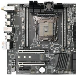
The EVGA X299 Micro ATX 2 Motherboard This motherboard contains the Intel® X299 chipset.
