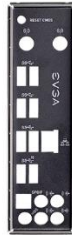
I/O Shield Installs in the system case to block radio frequency transmissions, protect internal components from dust, foreign objects, and aids in proper airflow within the chassis.
