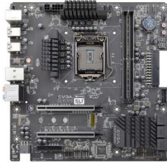
The EVGA Z370 Micro ATX Motherboard This motherboard contains the Intel® Z370 chipset.
